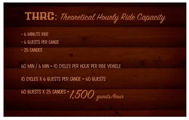
Figure 14. Theoretical Hourly Ride Capacity (THRC) Calculation
